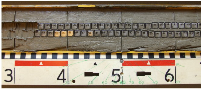
Fig. 2. Sampling of the cores. Two rows of 1 cm 3 cubes are pushed into the sediment; the two rows are offset by half a cube to increase the sampling resolution. Yellowish colors on some cubes is light reflection. The sample cubes were numbered row by row from top to bottom of the core. To reduce oxidation of the sediment, the small holes in the plastic cubes were sealed with acid-free silicone paste and the samples were stored in the fridge.
